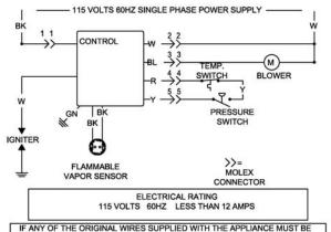
MINIMUM TEMPERATURE RATING OF 105°C AND A MINIMUM SIZE OF NO. 18 AWG. Figure 6
