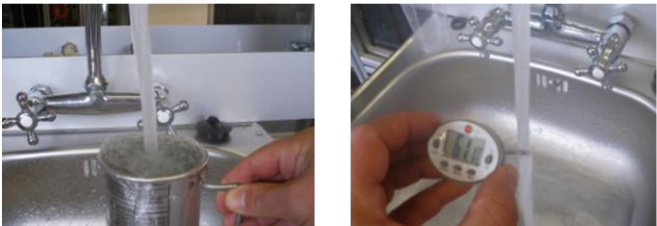
Figure 6 – Use of Water Flow Meter and Thermometer
