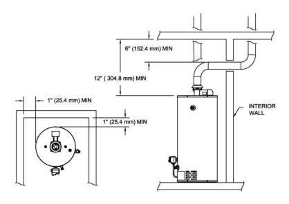
Figure 1. Minimum Clearances for an Alcove Installation.
