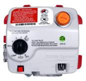
This new ICON System® control is the first of its kind offering built-in field convertibility. The control includes a regulator, located behind the orange cap, that is used when the water heater needs to be field converted from LP to natural gas. The water heaters themselves also ship with the alternate orifice and pilot assembly - no additional parts needed for fuel conversion!
