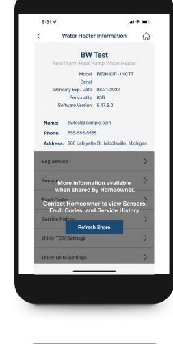
contractor can remotely see sensor information, previous service logs, and specifically what error messages have been triggered on the appliance, if any. Essentially, the contractor can access the water heater diagnostics the same as if they were in the room with the Bradford White Connect™ compatible heater and used the Service Existing Water Heater function on the contractor app.
