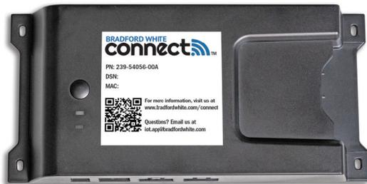
For spacing, the Adapter must be within 5 feet of a 120V outlet and must be within reach of the ethernet port on the front of the water heater. The supplied ethernet cable is 7 feet long, however an ethernet cable (CAT5e) up to 100 feet long will work as well. The action button and front label of the Adapter must be visible and easily accessible during installation.
