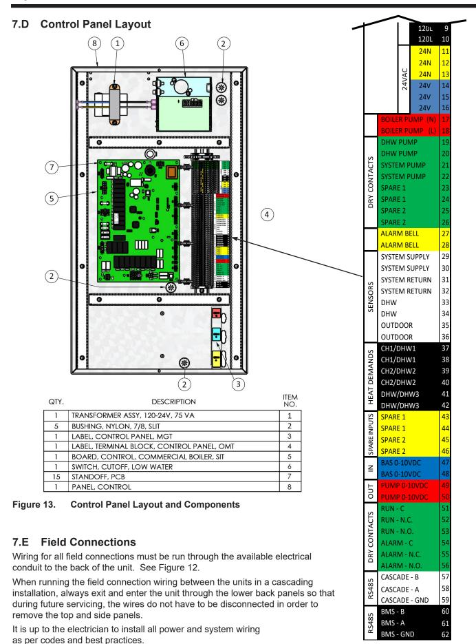
Figure 14. Field Connections (on Terminal Block 1)
