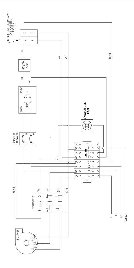
Figure 19. Wiring Diagram, 208V 3 Phase 2500
