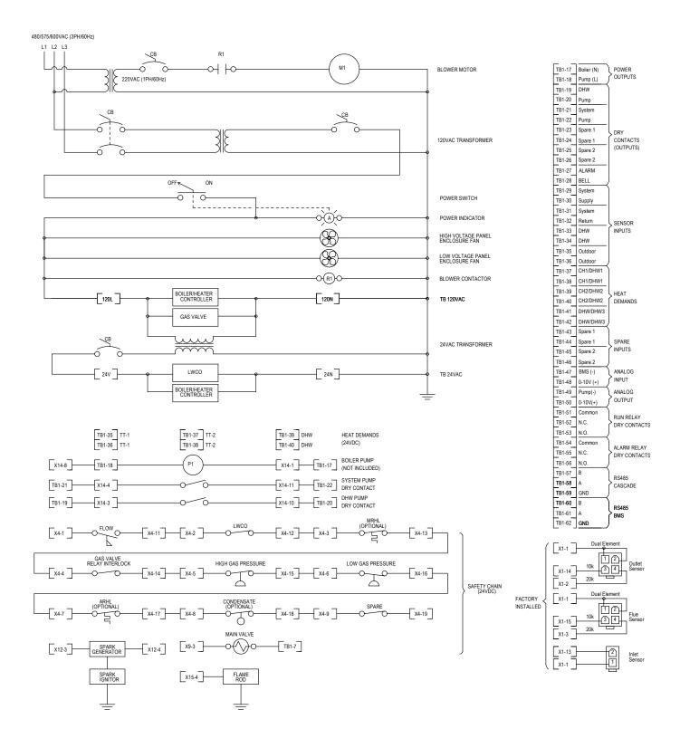
Figure 24. Logic Diagram 480, 600V 3 Phase 2500
