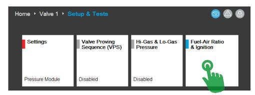
**Fuel Air Ratio & Ignition** has several menus that allow for combustion setup, Ignition characteristics modification, Loading and saving A/F curves and valve configurations.
