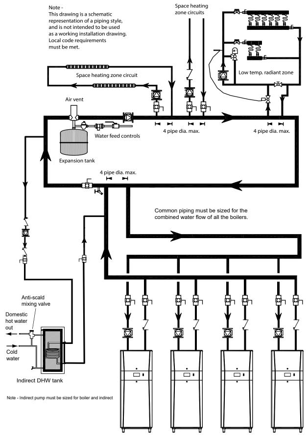
Figure 6. Boiler Piping — Multiple Boilers, Multiple Temperature Zones, Reverse Return.
