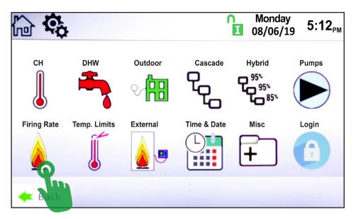
Boiler display>Configure>Firing rate. Force the fan speed to the desired RPM by navigating through the boiler display and setting the Fan RPM. Enable fan speed and set the fan speed to desired RPM. Use the following RPMs to set combustion, 1000, 1500, 2000, 3000, 4000, and maximum fan speed.
