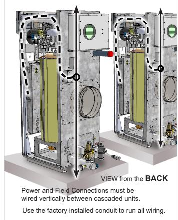
Figure 12. Wiring Access
