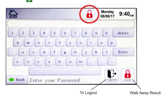
**Logout.** If the Installer is done and wants to lock the display immediately, tap the Logout icon to exit Installer or User Mode. Exiting the Installer or User Mode will lock the unit.
