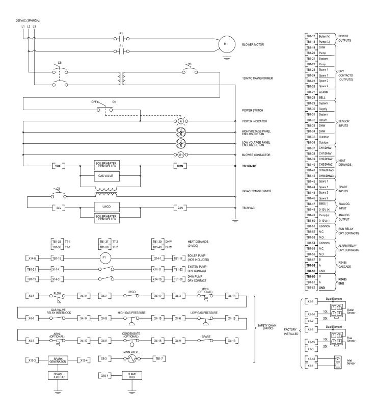
Figure 22. Logic Diagram 208V 3 Phase up to 2500
