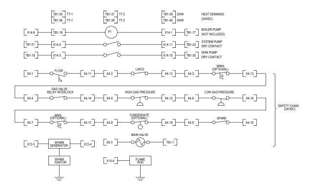
Figure 21. Logic Diagram 120V 1 Phase up to 2000
