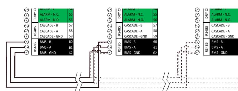
Figure 16. BMS Wiring Connections
