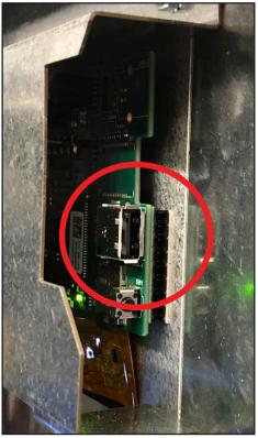
Figure 30. Photo of USB Slot on the back of touchscreen display.
