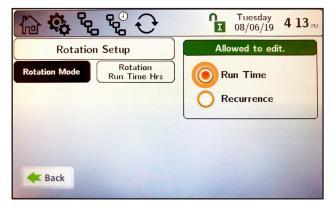
In the **Run Time** Mode, you can adjust only the Rotation Run Time Hours. This chooses which unit will fire first based on run time hours.
