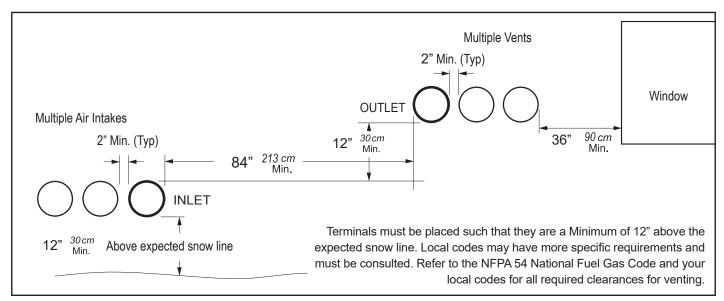
Figure 3. Minimum Venting Distance for Single and Multiple Units.
