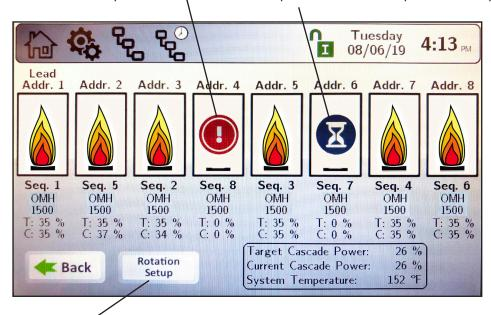
The Rotation Setup button is found only on the boiler that is assigned as 'Lead' and appears only when the lead boiler is in the Installer Mode.
