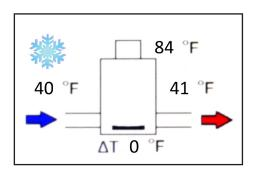
Figure 29. Active Anti Frost Condition
