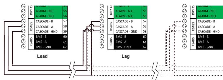
Figure 15. Cascade Wiring Connections
