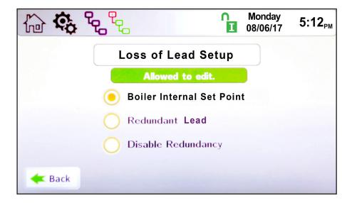
Note: The redundant lead unit should have a system sensor and be connected to the system pump (if / where applicable). In cascade if the lead boiler looses the system sensor, it will turn on the system pump but shut off the cascade communication. The Cascade will respond by the Redundancy settings setup by the installer.
