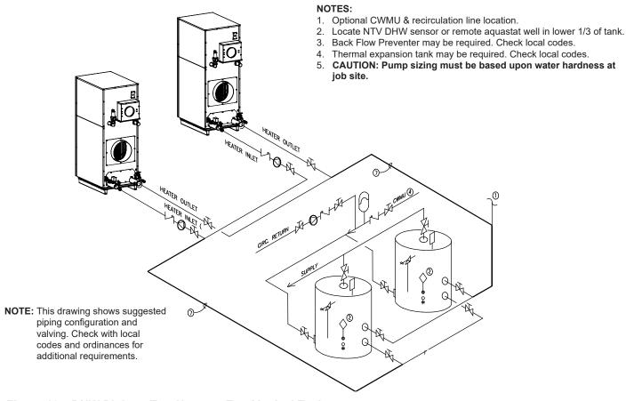
Figure 10. DHW Piping - Two Heaters, Two Vertical Tanks
