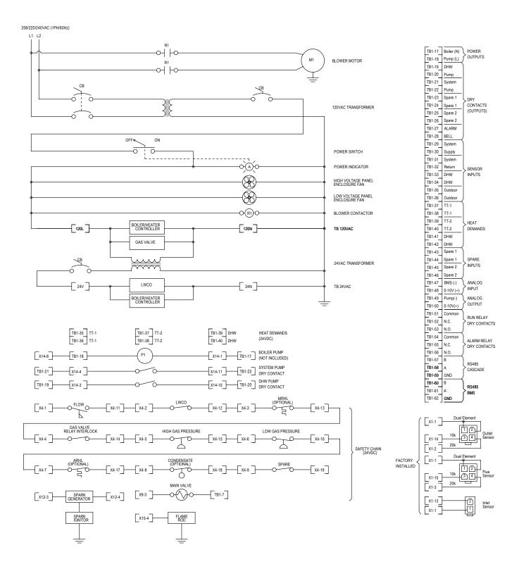
Figure 23. Logic Diagram 220V 1 Phase 1500 to 2500
