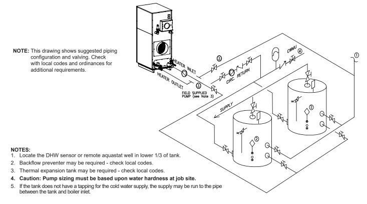
Figure 9. DHW Piping - One Heater, Two Vertical Tanks
