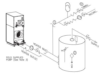
Figure 8. DHW Piping - One Heater, One Vertical Tank
